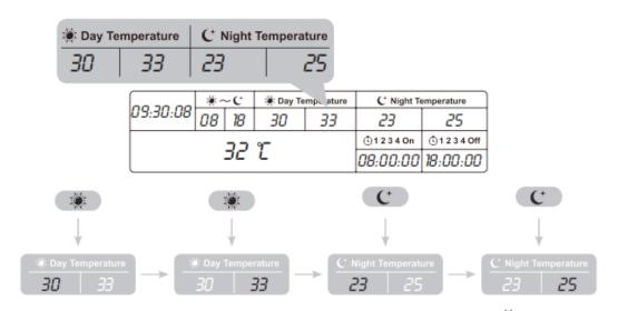
When the first value is less than the second value under the symbols "Day Temperature" and "C' Night Temperature", it means heating mode.
